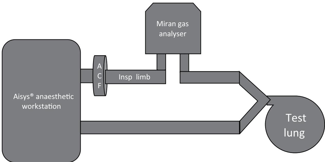
Figure 1: Diagram of anaesthetic circuit with the Miran gas analyser in series. ACF=activated charcoal filter.
